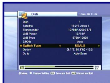
Go to Position : Press the
