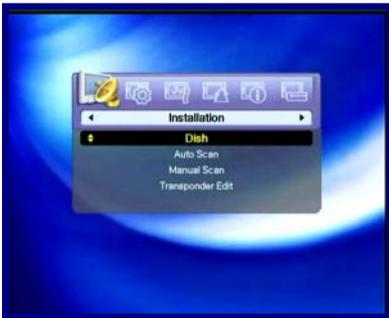
Press the MENU button to display the main menu. You can select the sub menu using the ▲/▼/◀/▶ button. The selected sub menu becomes highlighted. When you have selected the sub menu you want, press the **OK** button. When you want to return to the previous menu, press the **EXIT** button. When you want to return to the live screen, press the Menu button.
