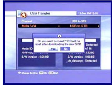
1. The window will appear on the TV screen if the data exists in the target. If you select "Yes", the data will be transferred. The window will appear on the TV screen while the data being transferred. You should keep USB connection until transferring is done.
