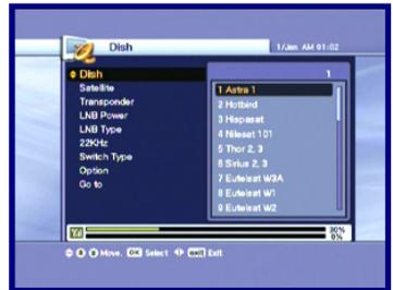
1. Press the **◀/▶** button to watch the satellite in the pre-programmed lists. Press the **OK** button to replace the Current satellite with the selected satellite.
