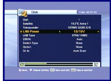
1. Select the LNB Type value. If you have selected User Single or User Dual, enter LNB frequency value directly, and press the OK button. If you select LNB Type value as 9750/10600, 9750/10750 or User Dual, 22KHz value is fixed to auto mode, in other case you can select a value depending on usage of 22KHz tone switch box.
