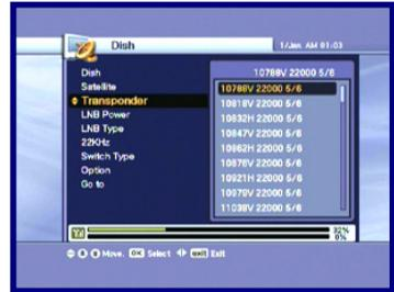
1. Select one of the LNB Power types using the ◀/▶ button. You can select LNB Power value as 13/18V normally or if the distance between antenna and receiver is further than 60m, you can select LNB Power value as 14/19V.
